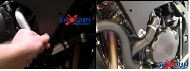
5. Remove the bodywork and double check location of spot mark the tool has created.
