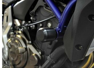
3) Slide the plastic slider over the top of the base and secure it in place using the 8 mm countersunk bolt provided. The bolt passes first through the non threaded hole and then screws into the threaded hole on the far side of the base. The plastic is undersized on the far side of the slider to act as a locknut for the bolt.
